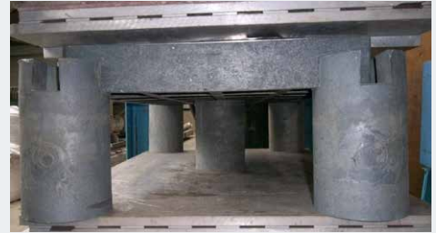
The stability of the structure after 48 hours at a load of 60 tonnes/m 2 (12,289 lbs/ft 2 ).
